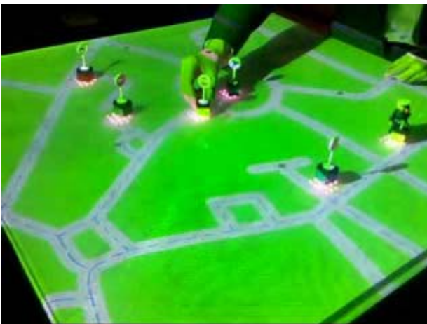
Figure 2: The Tangisense table used in a road traffic simulation application. One distinguishes tangible objects (e.g. road signals) and virtual objects video-projected (e.g. roads).
