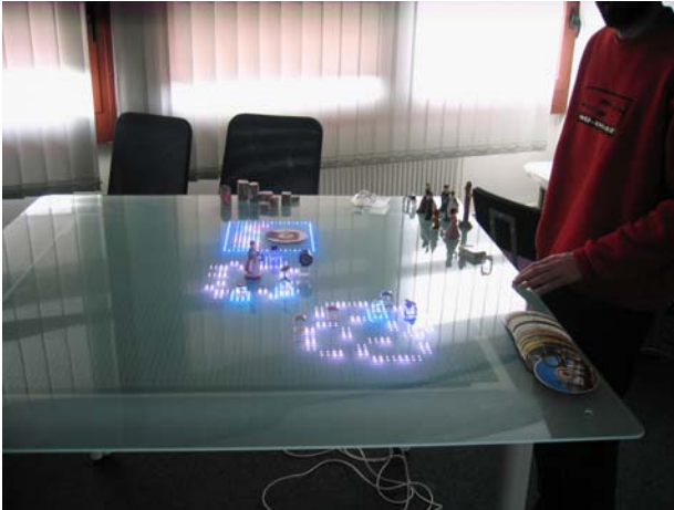
Figure 1: The Tangisense table under a configuration of musical creation. Bright areas (LEDs in the table) are activated by tangible "characters". A cube in the foreground is a musical instrument; a CD in the background is a database of sounds that can "dump" on the table.
